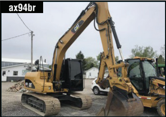
10 CAT 312D 4,502 hrs., 97 hp, Cab Aux Hydraulics, Quick coupler, Good UC 28" pads..... $81,500
