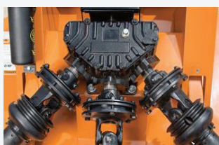
210 HP Rated Gearbox w/ Slip Clutch
