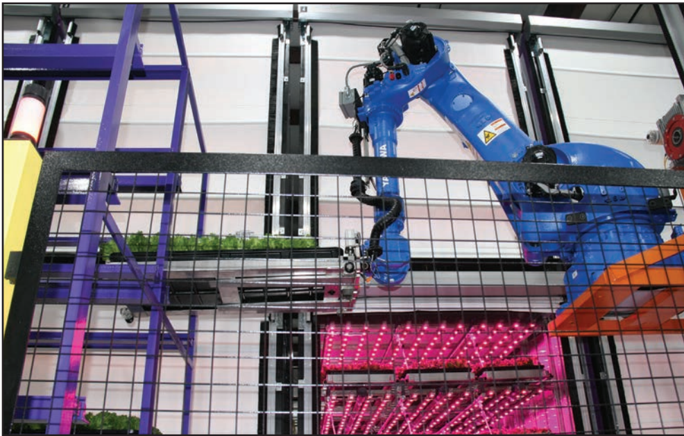
Above: 80 Acres is an indoor farm with robots doing the heavy lifting. They use LED lights, only the blue and red spectrum, which is what plants need and why photos look pink. The growers come up with the perfect light recipe for each plant.
