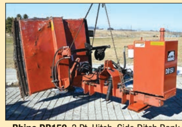
Rhino DB150, 3 Pt. Hitch, Side Ditch Bank Mower, Hyd. Driven 540PTO, Call
