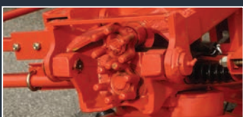
Exclusive DigiDrive® couplers provide low maintenance and long life
