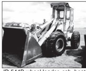
JD 544B wheel loader, cab, heat, turbo, coupler, 105 HP, 2 yd bucket . . . . . \$12,900
