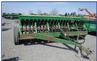
GP SOLID STAND 13 GRAIN DRILL, Stk. #3761, 13', end wheel, 1990yr, 7.5"sp, grass, only 2200 acres, one owner . . $6,950
