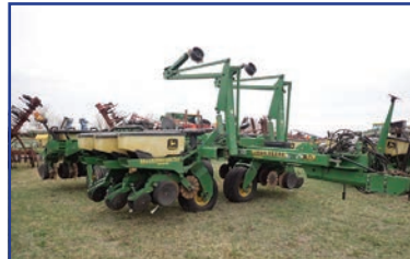
JD 1780 PLANTER, Stk. #3798, 12/23R, VAC, NT, keeton firmers, computrak 250 monitor, 3bu boxes . . . . . $19,500
