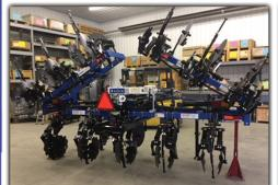
Very nice DMI 11 shank machine, field ready. Complete tear down, every bolt, nut & part taken off. Blasted & powder coated. All new bearings, blades, knives, hoses & coupler. Ravens has been rebuilt, resealed & tested ok.
