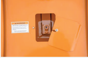
Quick Change and Greaseable Blade Pins
