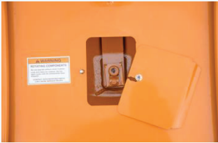
Quick Change and Greaseable Blade Pins
