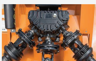
210 HP Rated Gearbox w/ Slip Clutch
