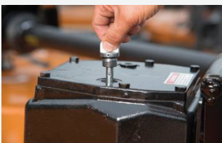
Gearboxes with Dipsticks and Drain Plugs
