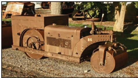
Above: Found in this museum is this 1938 Buffalo-Springfield tandem roller, which weighs five tons. (photo submitted)
