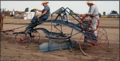
Above: The teamster would sit up front and the blade man stood in back on this 1920 Austin Standard pull grader. (photo submitted)
