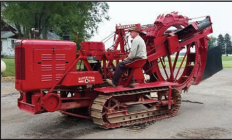
Above: Cleveland Trencher Company's main product was wheel trenchers, like this 1953 model 140. The 'wheel' is the structure carrying the buckets. It is lowered into the ground to dig a trench. (photo submitted)
