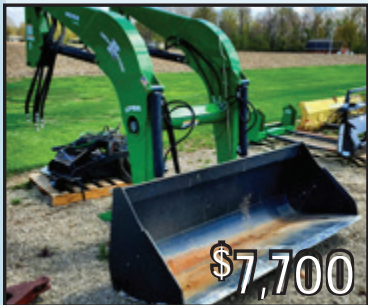
WOODS LF 156 LOADER 7 FT QT BUCKET, 3 HYD, JOY- STICK CONTROL, OFF JD 4450
