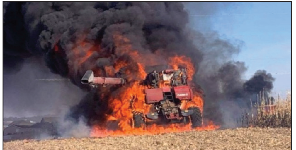
Above: Common causes of combine harvester fires are crop residue build-up, lubricant or fuel leaks, mechanical and electrical failures, a poor maintenance schedule and a lack of prevention plans.
