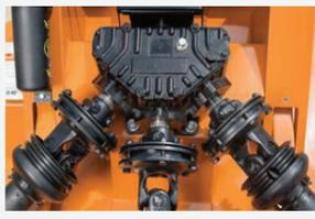
**210 HP Rated Gearbox w/ Slip Clutch**
