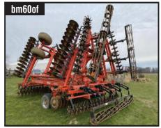
KUHN KRAUSE 8000-30' Excelerator, round bar reel, walking tandems, hydraulic down pressure . . . . . . . . . . . . . . . . . \$49,500
