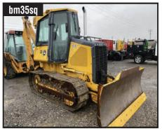
2005 DEERE 550J LT Only 2,635 hrs, full cab with heat & A/C, 6 way blade, joystick
