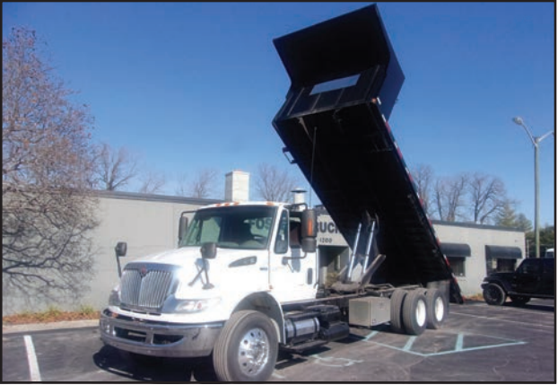
2013 INTL 4400 , INTL MF9, 315HP, 10SPD, SPRING SUSP, P/S, A/C, 292WB, 24' FLATBED DUMP, 11X22.5, 203,050 MILES . . . . . $43,500
