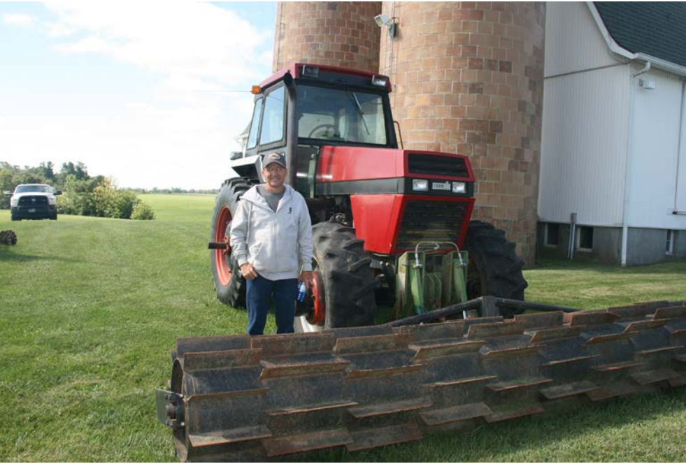
Above: Chris Proeschel and his son, Alex, designed and built this cover crop crimper. They started with a big pipe from a well-driller and improvised.
