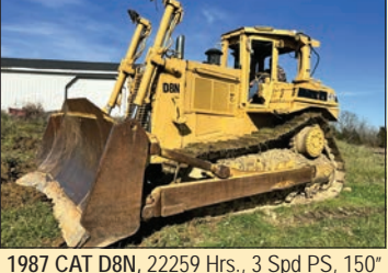
1987 CAT D8N, 22259 Hrs., 3 Spd PS, 150" Semi U Blade, 72" Pads, Hitch, $64,500
