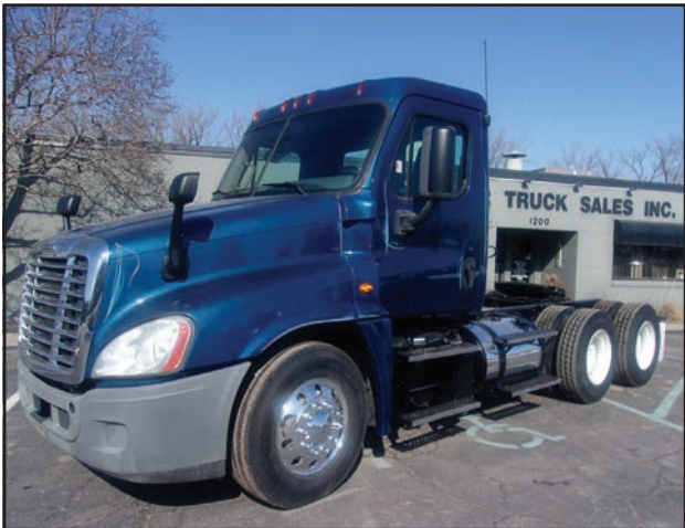
2015 FREIGHTLINER CASCADIA DETROIT DD15 455HP ENGINE BRAKE 10SPD AIR RIDE SUSPENSION P/S A/C POWER WINDOWS & LOCKS 178WB 11X22.5 ALUMINU 267,169 MILES. . . . . $44,500
