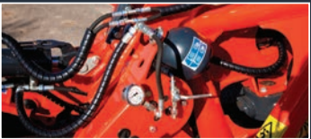
Lift-Control hydropneumatic suspension minimizes ash incorporation
