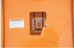
Quick Change and Greaseable Blade Pins
