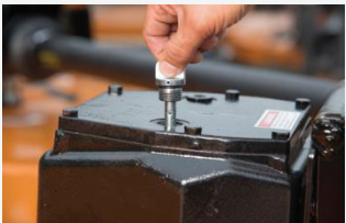
Gearboxes with Dipsticks and Drain Plugs
