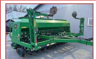
2000 JD 1560, 15' width, 2 pt factory hitch, factory JD markers, drill fill, excellent quality!! . . . . . $32,900
