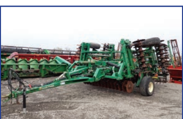
GP 1800TM TILLAGE TOOL, stk#2604, 18', weight kit, rockflex, spike harrow w/ crumbler, hyd angle, sharp . . . . $38,500
