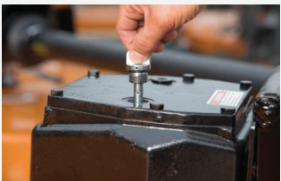
Gearboxes with Dipsticks and Drain Plugs
