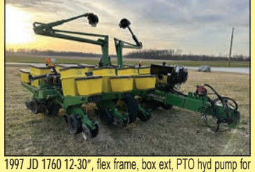
1997 JD 1760 12-30", flex frame, box ext, PTO hyd pump for vac, monitor & manuals, JD 250 monitors & Ag Express speed sensor, precision corn meters, JD soybean discs. $24,900
