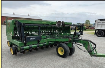
JD 750, 15' no-ill drill w/grass seeder attachment & markers, 7.5" spacing, good used drill .. $19,500
