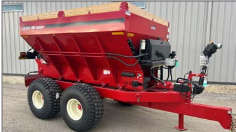
New Stainless BI Liberty 10 Ton Hopper Variable Rate Lime/Fertilizer Spreader
