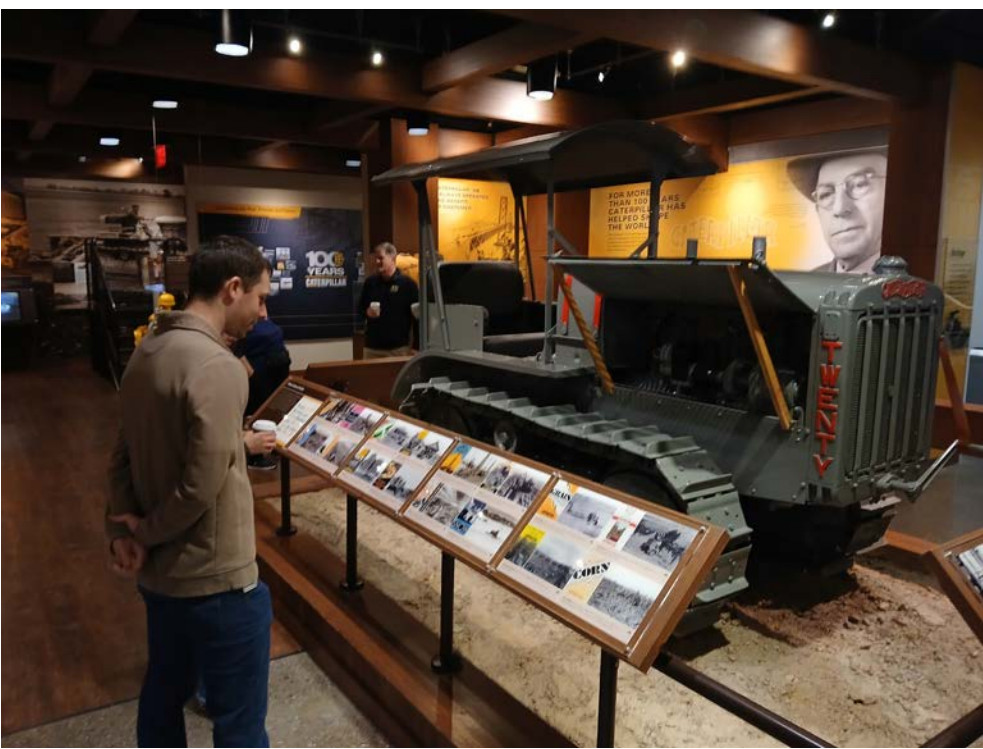
Above: A CAT Visitors Center guest is pictured checking out a vintage CAT 20 tractor. The Model 20 was the first product designed and built by CAT that was not a carryover from Holt or Best. It was introduced in 1927 in San Leandro, Calif., then began production in East Peoria a year later. (All photos by T. Alexander)
