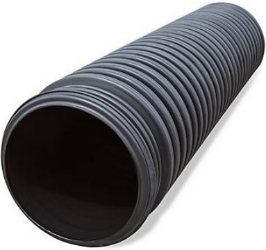
Above: Dual wall tile has a corrugated exterior for strength, and a smooth interior for better flow. (photo provided)
