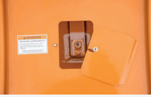
Quick Change and Greaseable Blade Pins
