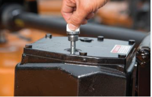
Gearboxes with Dipsticks and Drain Plugs
