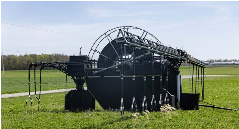
Above: Pictured is the 360 RAIN unit, an autonomous irrigation system designed to deliver water, nutrients and even manure to crops only where needed. The sprayer utilizes water/nutrient only as needed and helps prevent runoff. (photo submitted)
