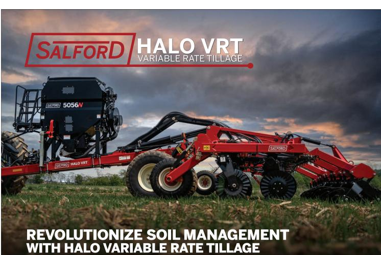
Salford's HALO VRT adapts to your soil's needs. Adjust blade angles hydraulically from 2 to 15 degrees, changing to meet varying soil conditions from field to field and season to season.
