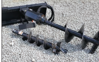
Jenkins posthole digger, 2" hex drive, 9" & 18" augers..... $3,100
