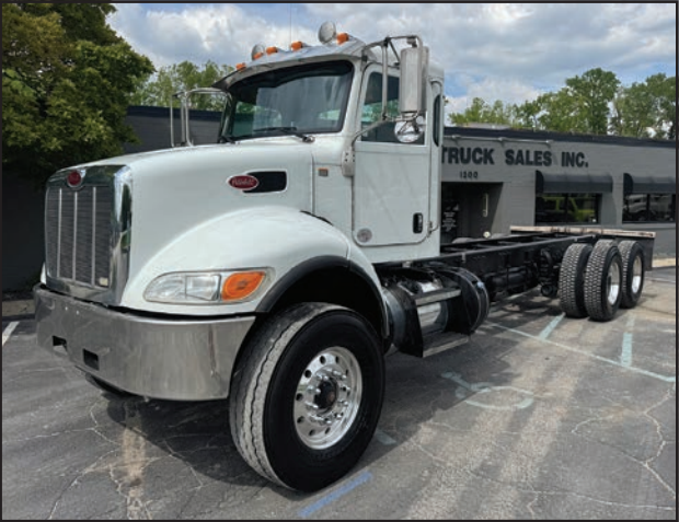
2020 PETERBILT 348 PACCAR PX9 370 HP ALLISON 3000RDS PTO PORT TRANSMISSION AIR GLIDE SUSPENSION 20,000 FRONT AXLE P/S A/C 235WB 315X22.5 FRONT TIRE 11X22.5 REAR ALUMINUM BUDDS. . . . . 157,025 MILES - $ 89,500
