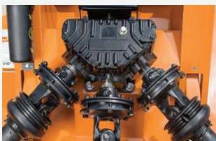
210 HP Rated Gearbox w/ Slip Clutch
