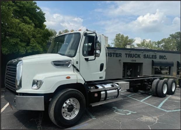
2017 FREIGHTLINER 114SD DETROIT DD13 450 HP EATON FULLER FRO-15210C TRANSMISSION 46,000 TUFTRAC SUSPENSION 18,000 FRONT AXLE P/S A/C FULL LOCKERS DOUBLE FRAME 4:11 RATIO 288 WHEEL BASE 315X22.5 ALUMINUM BUDDS FRONT 11X22.5 STEEL BUDDS REAR. . . .388,803 MILES SOUTHERN TRUCK $69,500
