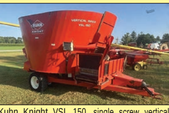
Kuhn Knight VSL 150, single screw vertical mixer, set up as left hand discharge, small 1000rpm, inline walking tandems, scale ..... $23,500
