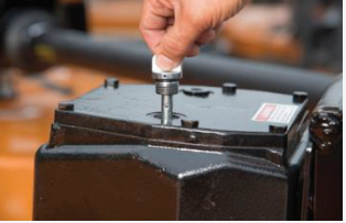
Gearboxes with Dipsticks and Drain Plugs
