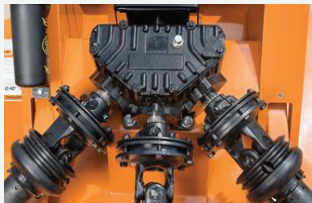
210 HP Rated Gearbox w/ Slip Clutch
