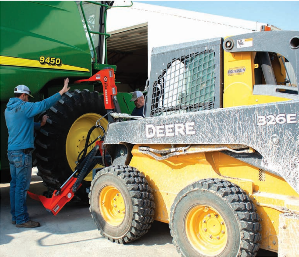
Above: Nathan Meyers, manager of Iowa State University’s Agricultural Engineering and Agronomy Farm, uses the TireGrabber to change the front tire of a combine. (courtesy of Iowa State University College of Agriculture and Life Sciences)
