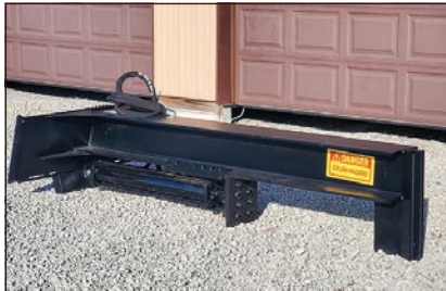
Jenkins wood splitter, 5" 30-ton cylinder, 36" bite..... $3,200
