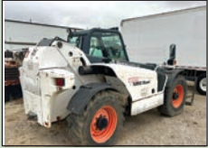
2008 Bobcat V723, Enclosed Cab, 23' Max Lift Hght, 7000 Lb Max Lift Cap., 48" Hyd. Coupler, Frame Leveling, Aux. Hyd. Plumbing, 400/80-24 Tires... $27,500
