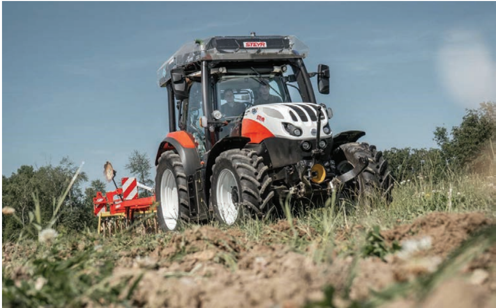
Above: STEYR & Tu Wien's hydrogen fuel-cell powered tractor.
