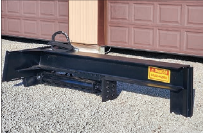
Jenkins wood splitter, 5" 30-ton cylinder, 36" bite..... $3,200
