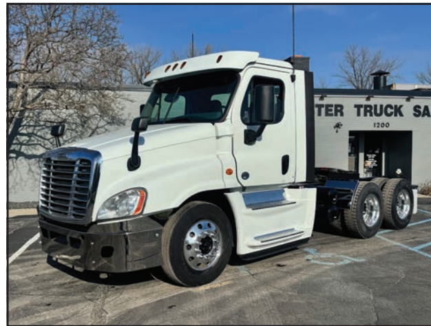
(5) 2019 FREIGHTLINER CASCADIA DET DD13 450HP ALLISON AUTOMATIC 4000HS TRANS AIR RIDE SUSP P/S A/C 3:70 RATIO 182WB 11X22.5 ALUM BUDDS 664,280 74,772 75,280 80,627 86,825 MILES . . . . . $62,500 EACH
