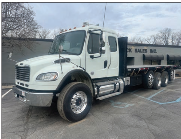
2020 FREIGHTLINER M2 106 EXTEND CAB CUMMINS L9 350HP ALLISON 3000RDS TRANSMISSION AIR RIDE SUSPENSION 16,000 FRONT AXLE P/S A/C 5:86 RATIO 2 LIFT AXLE 274 WHEEL 28' FLATBED 315X22.5 ALUMINUM BUDDS FRONT 11X22.5 ALUMINUM BUDDS OUTSIDE REAR . $79,500
