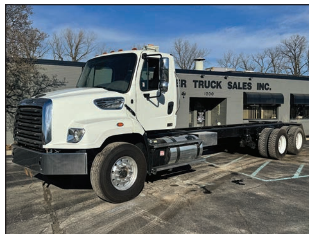
2017 FREIGHTLINER 114SD DETROIT DD13 450HP EATON FULLER FRO-15210C TRANSMISSION 46,000 TUFTRAC SUSPENSION 18,000 FRONT AXLE P/S A/C FULL LOCKERS DOUBLE FRAME 4:11 RATIO 288 WHEEL BASE 315X22.5 ALUMINUM BUDDS FRONT 11X22.5 STEEL BUDDS REAR 388,803 MILES SOUTHERN TRUCK. . . . . $59,500
