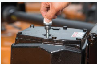
Gearboxes with Dipsticks and Drain Plugs
