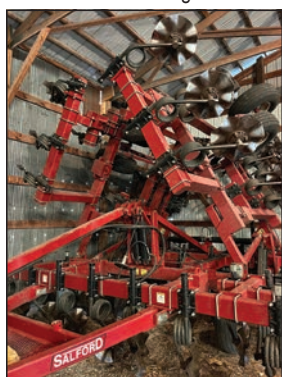
40' High Speed Disk- Notched Blades with Single Cage Roller
