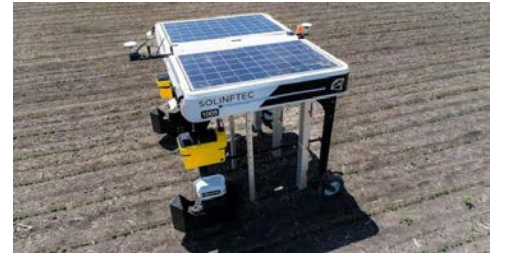
Above: The Solinftec solar-powered sprayer
