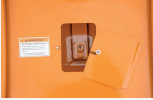
Quick Change and Greaseable Blade Pins
