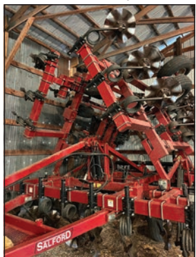
40' High Speed Disk- Notched Blades with Single Cage Roller
