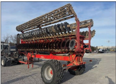
40' High Speed Disk- Notched Blades with Single Cage Roller
