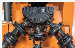
210 HP Rated Gearbox w/ Slip Clutch
