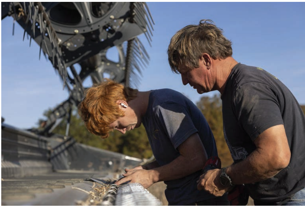
Above: Blake Gerard looks over the shoulder of his son, Wyatt, as the two repair damaged teeth on the header of their combine. (Lylee Gibbs photo)
