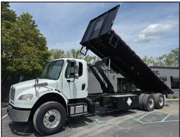
(2) 2017 FREIGHTLINER M2 106 CUMMINS 350HP ALLISON 3000RDS TRANSMISSION 44,000 AIR RIDE SUSPENSION 16,000 FRONT AXLE P/S A/C 5:86 RATIO 270WB 24' FLATBED/DUMP 315X22.5 ALUMINUM BUDDS FRONT TIRES 11X22.5 ALUMINUM/STEEL REAR TIRES . . . . . 189,573 MILES $89,500 212,824 MILES $88,500
