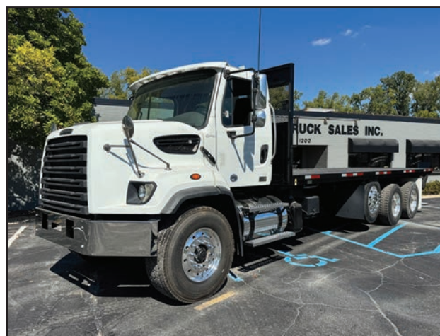
2 2016 & 2 2019 FREIGHTLINER 108SD CUMMINS ISL 370HP ALLISON 3000RDS TUFTRAC SUSPENSION 20,000 FRT AXLE P/S A/C LIFT AXLE 25' FLATBED 315X22.5 ALUM BUDDS FRT 11X22.5 REAR MILEAGE ..... 2016 303,251 $84,500 . 2016 210,029 $88,500 2019 120,159 $104,500 2019 64,125 $109,500
