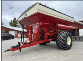
New 2023 Killbros 1035, 1000 bu. corner auger grain cart, 1050/50R32 tires, factory installed scales w/410 indicator, installed weather guard roll tarp. . . .CALL
