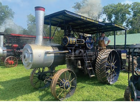
Above: This 1924 A.D. Baker & Company steam traction engine was built in Swanton, Ohio. The company was incorporated in 1901 to manufacture such engines, later expanding into large gas tractors. (Doug Graves photo)
