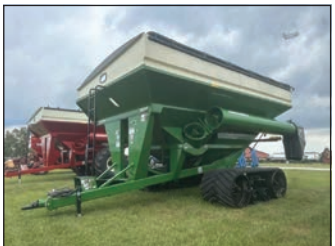
New 2024 Killbros 1035, tracks, 1000 bu., 20' corner aug, hyd. spout, factory installed scale pkg w/410 indicator & weather guard roll tarp, 36"x112' hyd tension tracked undercarriage . . . . CALL
