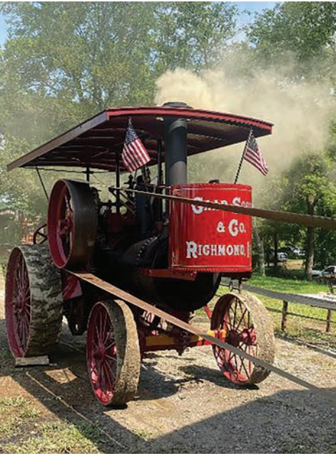
Above: The Garr, Scott & Co. was a steam engine manufacturer out of Richmond, Ind., from 1849 to 1911. This engine was hooked with pulleys and used to operate the saw blades during sawmill demonstrations. (Doug Graves photo)
